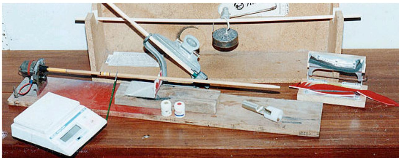
Clockwise from bottom left: Grain Scale, Cresting Jig, Fletching Jig, Spine Tester (at rear), Feather Chopper, Tapering Tool.
