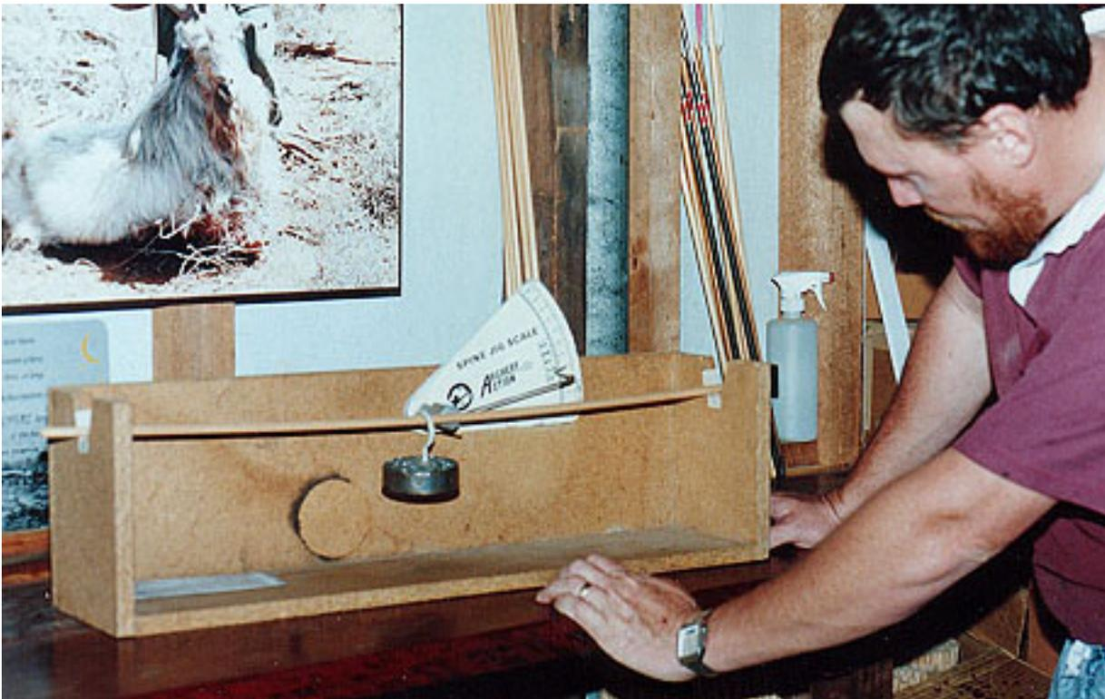
Using the spine Tester to find a shaft's spine rating.
